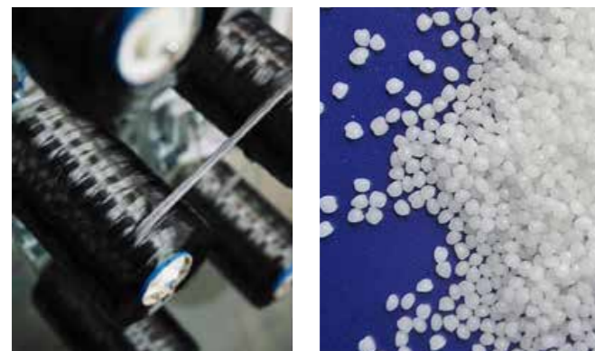
Left: Carbon Fibre on Coil / Right: Polymer Granulate
