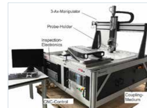
Construction and elements of the online-monitoring system at Fraunhofer ICT
