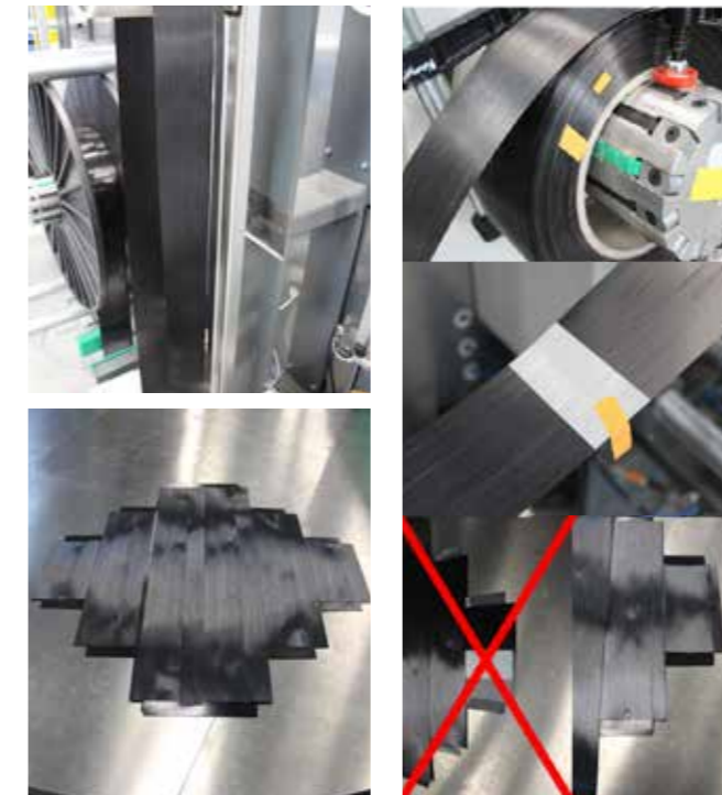
Left: Tracking defects to avoid passing them to the next value-added step. Right: Defect (gap) in tape is transferred into the tape layout
