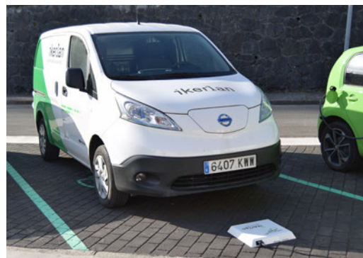
Wireless battery charger with an electric vehicle
