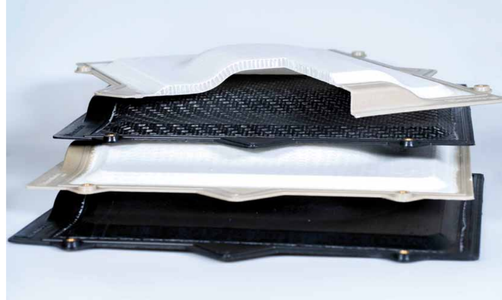
Test components produced in the thermoforming injection molding process, each made of different types of continuous fiber-reinforced sandwich composite.
