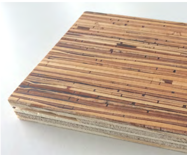
Laminate of birch bark layers and support plate
