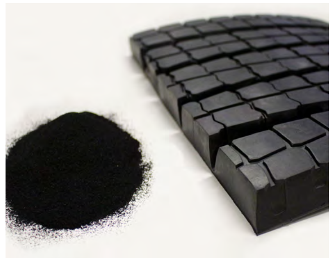
Example of our core competence in »microstructure design«: Composites optimized on the nanoscale ensure low rolling resistance for tires.
