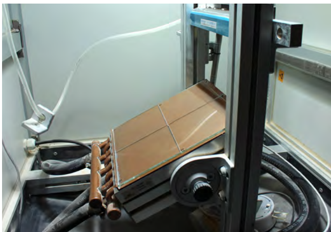
View into the dust chamber of the soiling test bench: Four dusty glass samples are bedewed here by cooling the sample table (detailed photo above).
