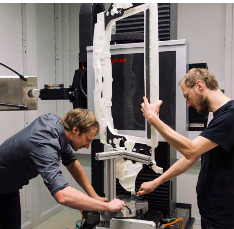
28 | In-situ x-ray computed tomography improves test methods for high-performance composites
