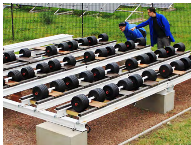
Long-term creep tests outdoors with inspection weights
