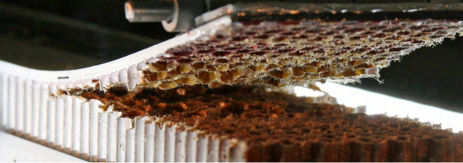
Sandwich sample in the single cantilever beam test: Facesheet depending at very high loads due to tearing of the aramid paper honeycomb core below the facesheet
