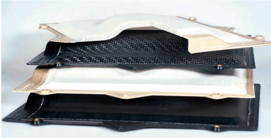
Fig. 3. Component demonstrators : 3D molded sandwich structure with injection-molded component edge, sawed component (top) and variation of the face sheet material (black components).
